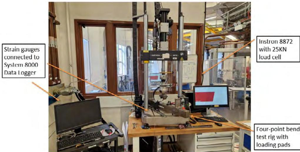
**Figure 2.** Experimental set-up for compression test of sandwich specimens.
