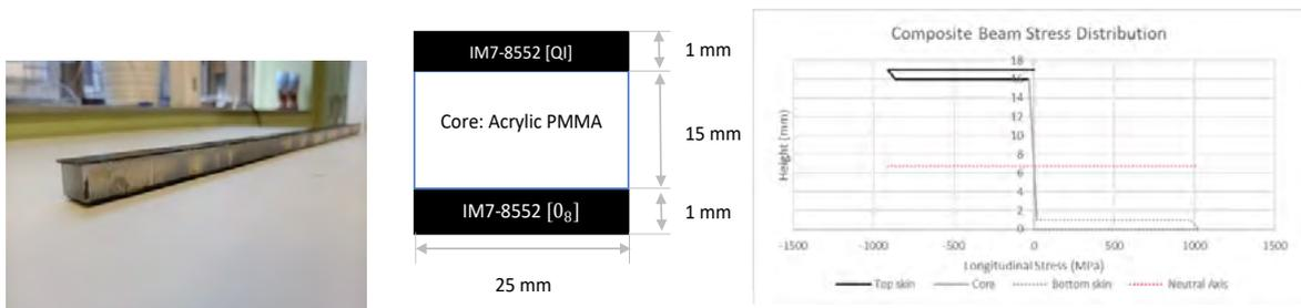
**Figure 1.** Composite sandwich structure (left), cross-section view of composite sandwich structure (middle), and composite beam stress distribution showing neutral axis for cross-ply sample (right).
