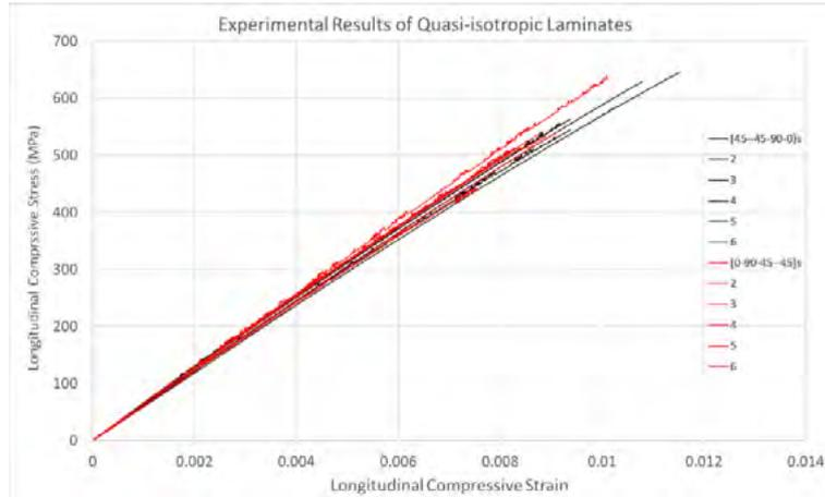
**Figure 3.** Experimental results of quasi-isotropic laminates showing two different stacking sequences.
