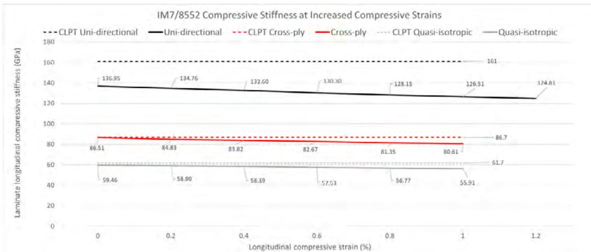
**Figure 5.** Longitudinal stiffness of quasi-isotropic, cross-ply, and unidirectional laminates at higher compressive strains.
