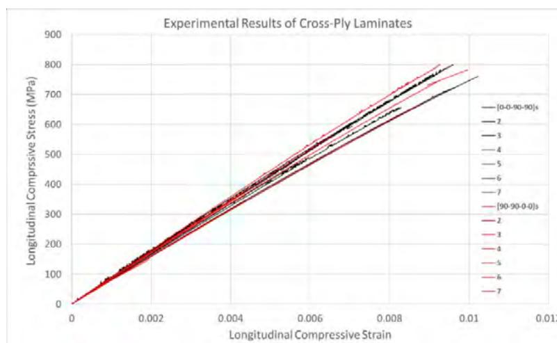
**Figure 4.** Experimental results of cross-ply laminates showing two different stacking sequences.
