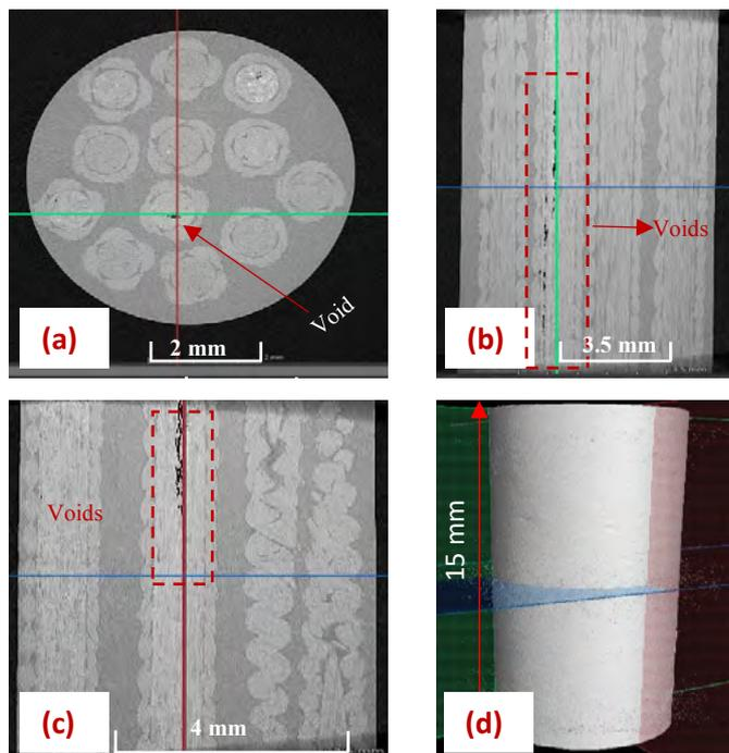
Fig. 7. Micro CT composite strut (manufactured @ $3 \times 10^5$  Pa) at 4 mm lay length and  $49^\circ$  braid angle showing (a) Top, (b) Front (c) Right and (d) 3D.
