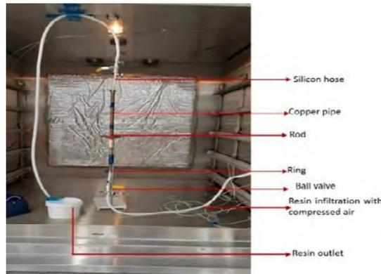
Figure 3. Manufacturing set-up for the over-braided composite struts with RTM
