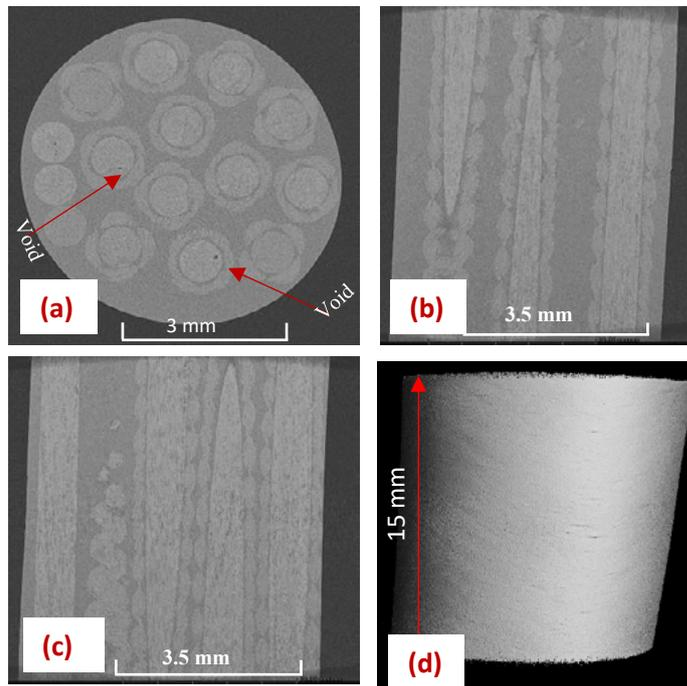
Fig. 8. Micro CT composite strut (manufactured @ $3 \times 10^5$  Pa) at 6 mm lay length and  $61^\circ$  braid angle showing (a) Top, (b) Front (c) Right and (d) 3D.
