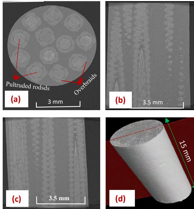
Fig. 6. Micro CT composite strut (manufactured @ $3 \times 10^5$  Pa) at 2.5 mm lay length and  $34^\circ$  braid angle showing (a) Top, (b) Front (c) Right and (d) 3D.
