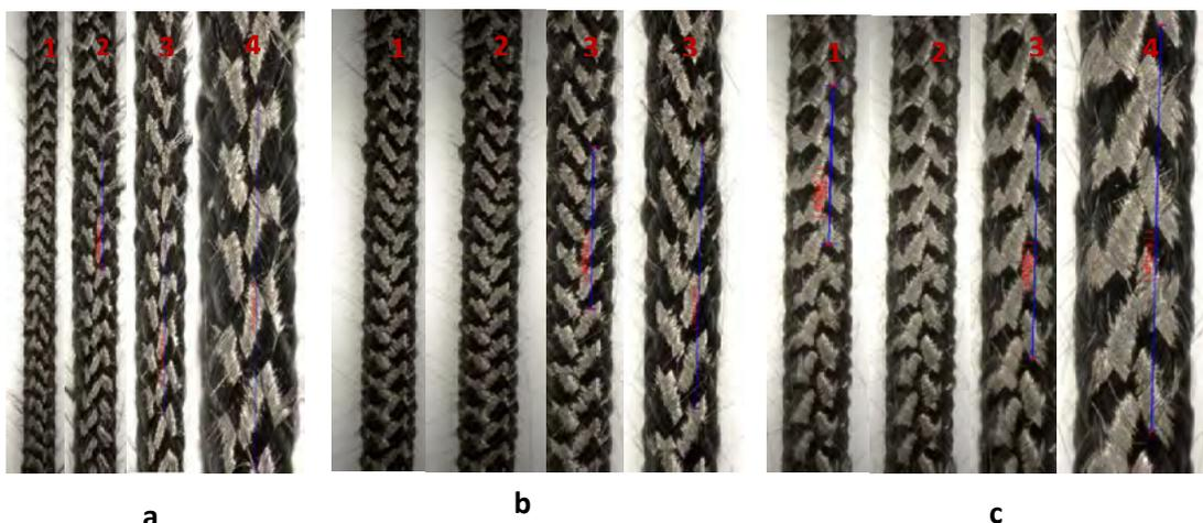
Fig. 5. Microscopic images showing fabricated overbraids at different lay lengths and magnifications for (a) 2.5 mm lay length (b) 4 mm lay length (c) 6 mm lay length at x20, x25, x30 and x40 magnifications
