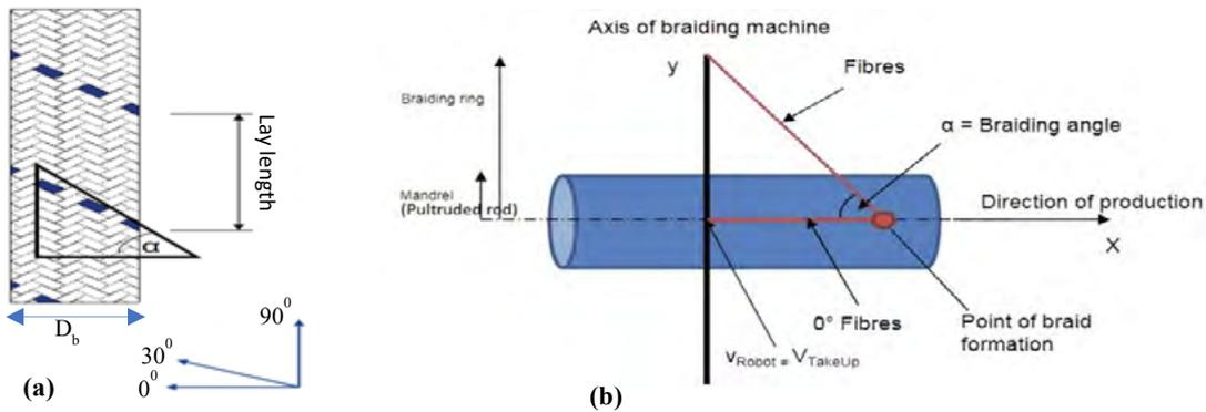
Fig 2. Schematic representation of (a) overbraid lay length and angles (b) geometric parameters in braiding adapted from [15].
