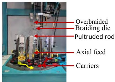
Fig 1. Herzog 1/16/80 circular maypole micro braider showing 8 carriers of Toray T300 carbon fibre
