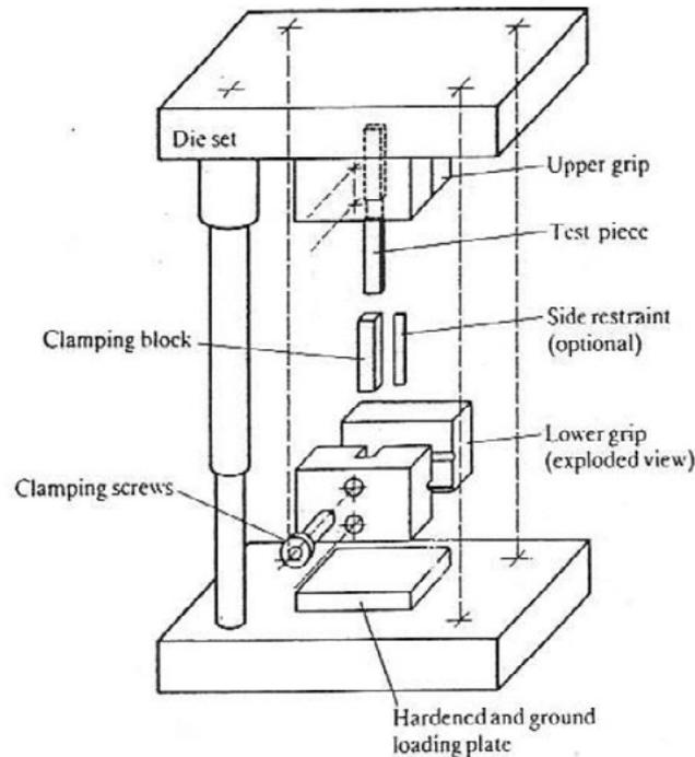
**Figure 2.** Imperial College Compression Standard fixture/test rig and specimen [14].
